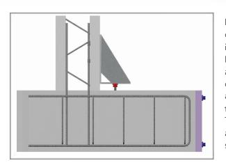
For the assembly and alignment of the double wall, adjusting devices are used. These allow an easy, fast and precise installation.
